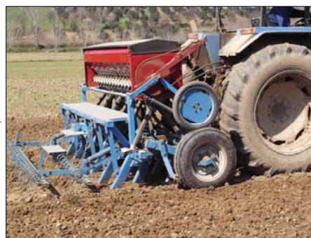
Seed drill Contemporary sowing of faba and wheat allowed by a double seed dispenser equipment.
